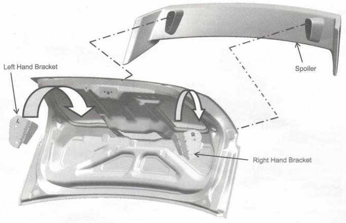
Insert the Left Hand and Right Hand Brackets in between the Inner and Outer Trunk Lid as shown
