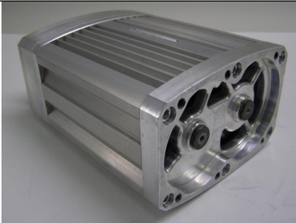
Rear view showing the intake plate / port
