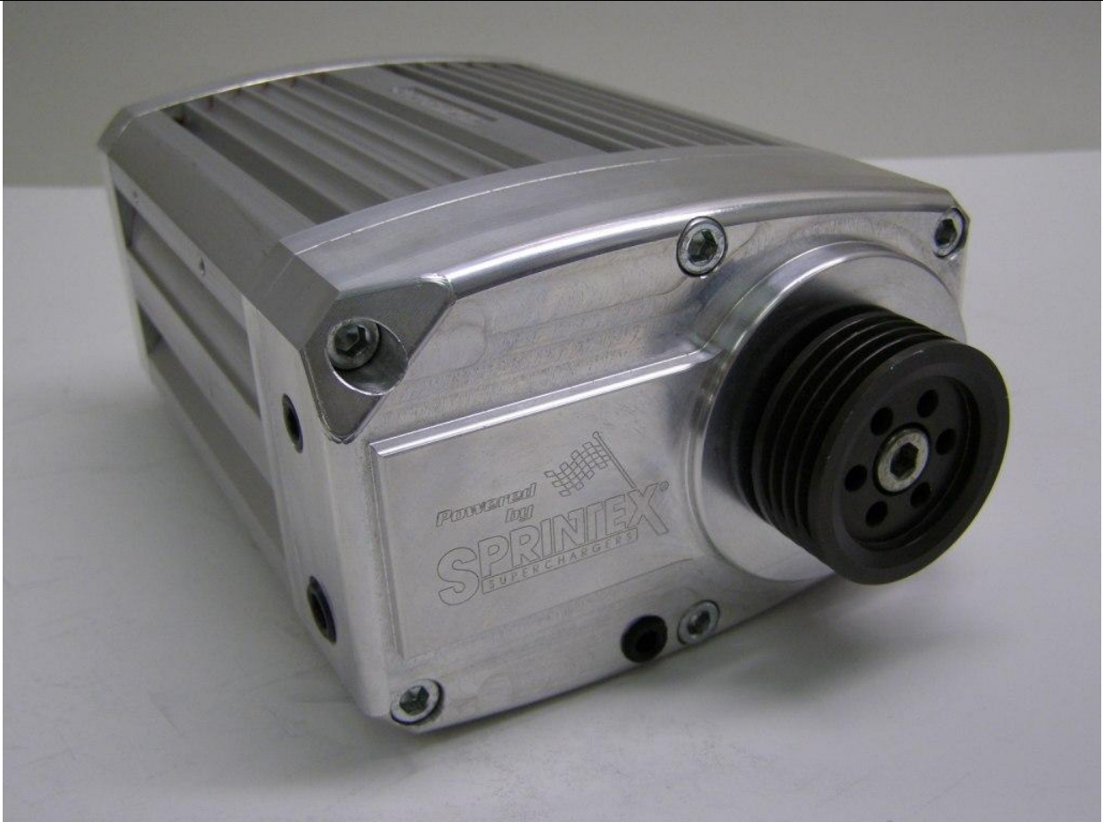
Front view showing the rotor pulley
