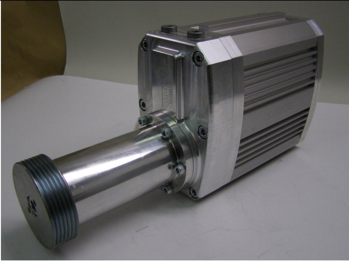
Front view showing the medium length extension housing with rotor pulley
