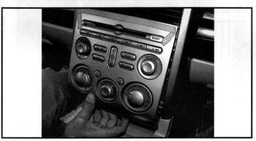
Connect the 2 harness connectors on the rear of the A/C Controller, fit the audio panel & A/C controller assembly.
