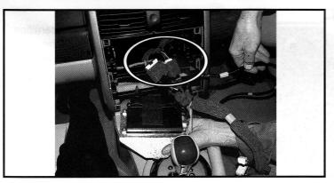
6. Plug in the 2 vehicle harness connectors to the kit assembly.
