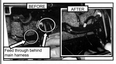
Locate the switch/mic harness identified in step 8 and feed it through to the driver's side foot-well area as shown.
