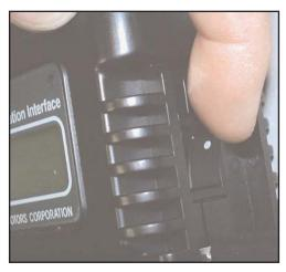
The VCI powersup in two ways: through the switch (the 16pin Diagnostic Connector has a 12-volt power feed) or through the Laptop (via the USB cable).
