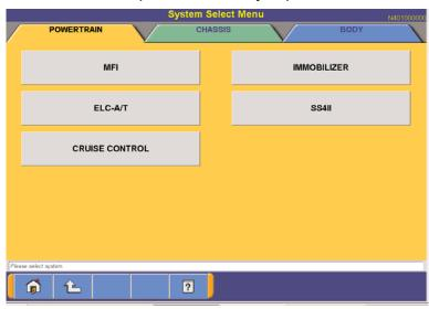
**System Select** provides you with 3 option tabs: POWERTRAIN, CHASSIS, and BODY
