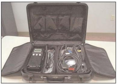
To connect the **S**can **T**ool **V**iewer to a vehicle, take the laptop, VCI, and the various adapter cables over to the vehicle. If you are going to use the A/C power adapter, make sure that you have a heavy-duty extension cord long enough to reach from the wall outlet to the vehicle. (The standard laptop battery lasts about 2 hours, but you can continue to use the Laptop while it is recharging.)
