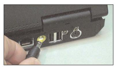
Plug the Laptop power adapter into a power strip and into the yellow outlet at the back of the Laptop.
