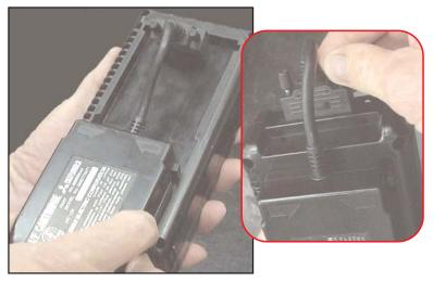
If you need the SWS Monitor Cartridge or Chrysler Powertrain Cartridge, attach it to the back of the VCI.
