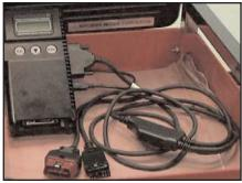
The VCI (Vehicle Communication Interface) connects the vehicle to the laptop computer.
